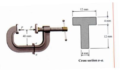
the combined axial and bending stresses, written in terms of the unknown P, can be set equal to the allowable normal stress. From these expressions, the maximum allowable clamping force can be determined.
