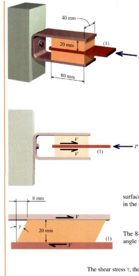
Two blocks of rubber, each 80 mm long by 40 mm wide by 20 mm thick, are bonded to a rigid support mount and to a movable plate (1). When a force of P = 2,800 N is applied to the assembly, plate (1) deflects 8 mm horizontally. Determine the shear modulus G of the rubber used for the blocks.
