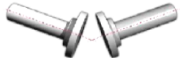
Angular Offset Misalignment
