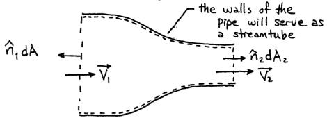
The vectors representing the areas (ndA) are directed outward from the control volume, as shown in the sketch. The velocities represent an assumed flow from left to right. Using the vector dot products and noting that the flow properties do not vary across the cross-section, we obtain:
