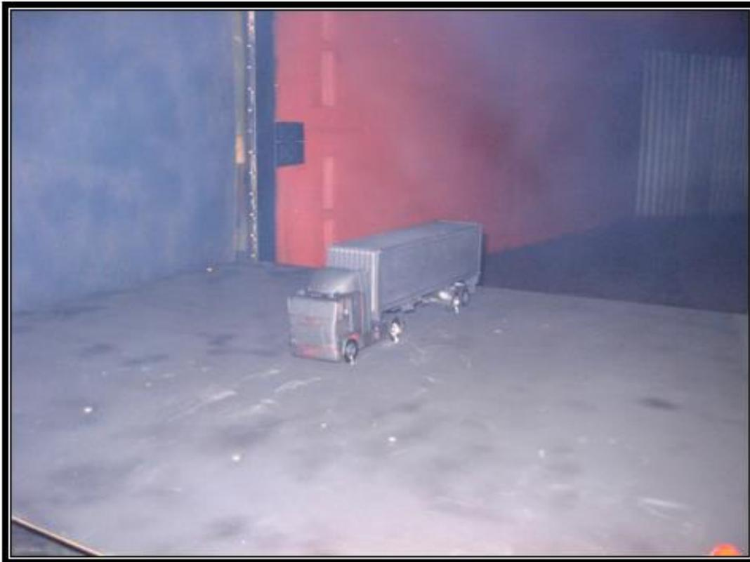
Picture #2 heavy-duty truck mounted on a plywood.
