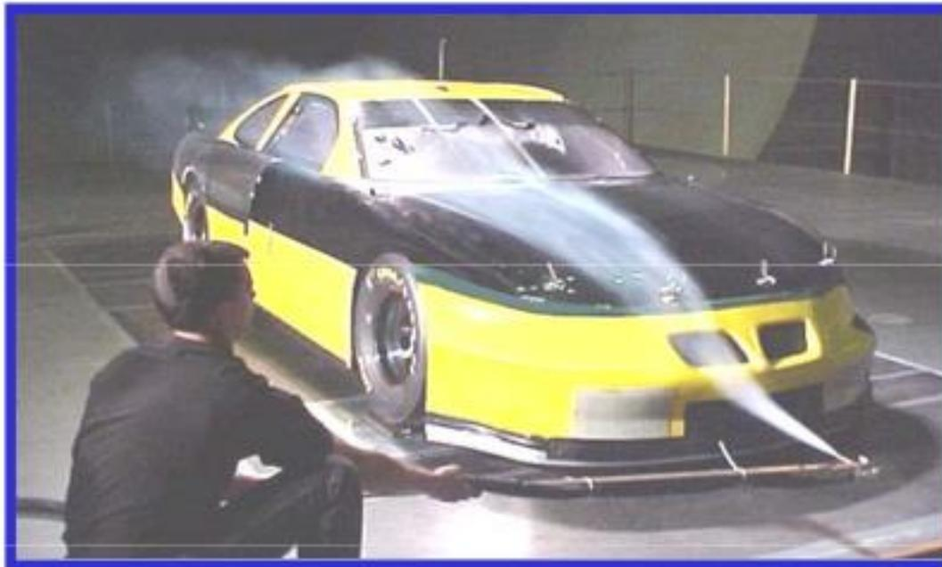
Wand used with full- scale automotive testing
