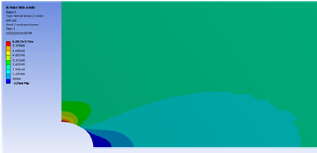
From this, you can see that most of the plate is in constant stress, and there is a stress concentration around the hole. The more red areas correspond to a high, tensile (positive) stress and the blue areas correspond to areas of compressive (negative) stress. Let's use the probe tool to compare the ANSYS simulation to what we expected from calculation. In the menu bar, click the Probe button; this will display the Sigma-x values at the cursor location as you hover over the plate.
