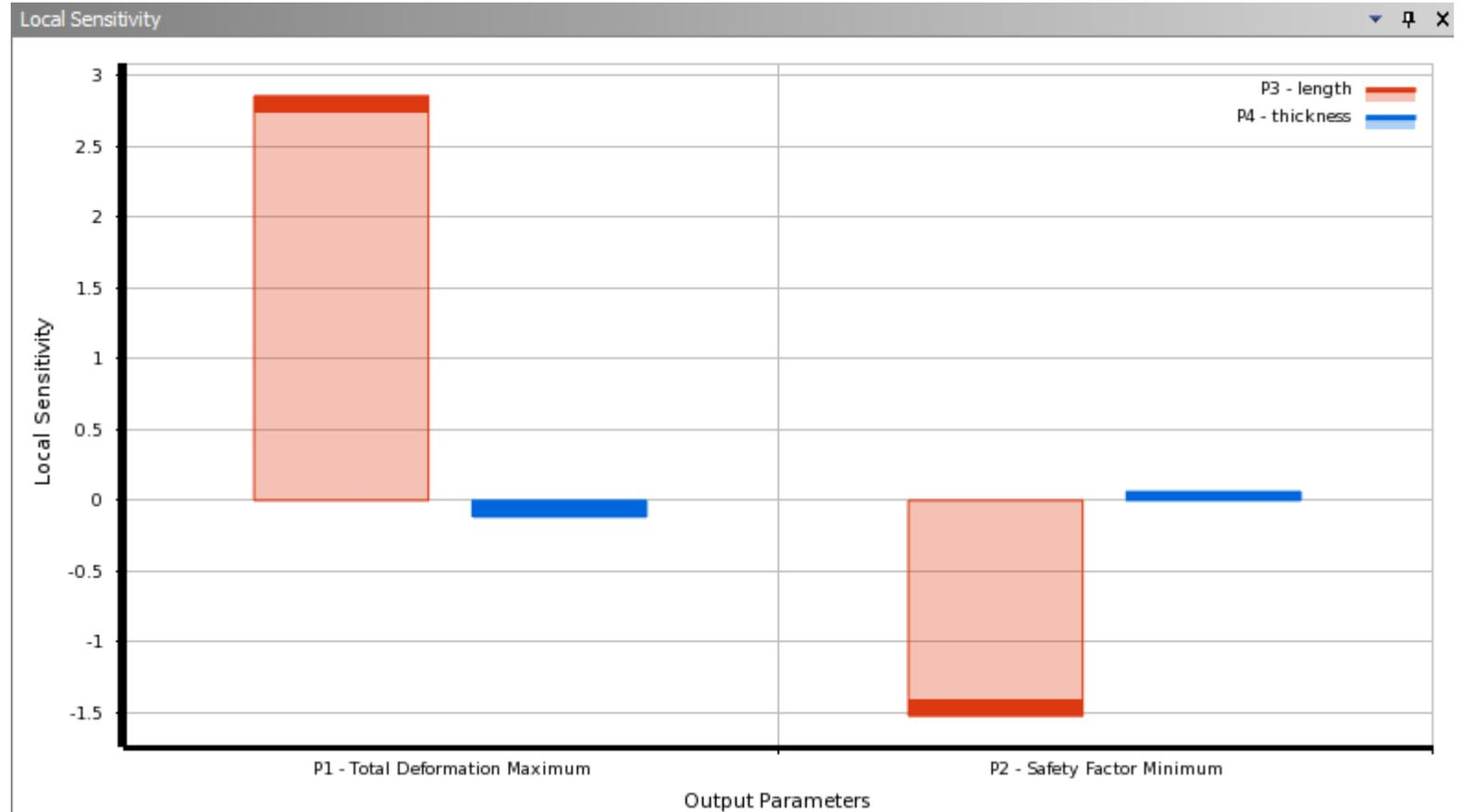
This plot shows how large of an impact each input parameter has on each output parameter at the current response point. It can be seen that length has a larger impact on both Total Deformation and Safety Factor at the center of our response surface
