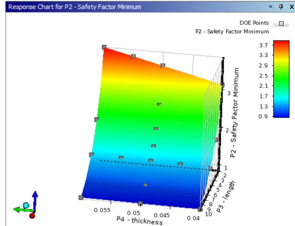
From the Response Surfaces, it is apparent that the gradient with respect to length is much larger than that with respect to thickness. To better resolve this gradient, the Sparse Grid method inserted more design points across the range of length values (9) than it did for thickness (5)
