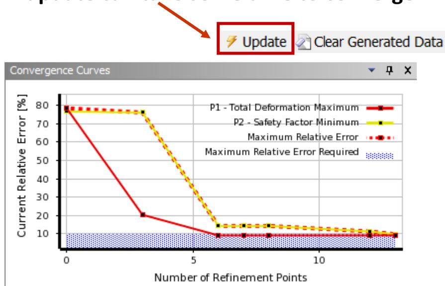
Here we can see the convergence of the response surface for each parameter. We can get more accurate response surfaces by decreasing the Maximum Relative Error, but more Design Points will need to be run to do so
