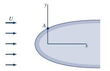
Write Bernoulli equation between stagnation point and point A to obtain  $\frac{p_{a}}{p_{a}} = \frac{p_{a}}{p_{a}} + \frac{1}{2} \rho V_{A}^{2}$
