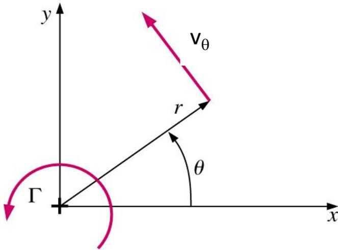
Equations are for a line vortex at the origin where the arbitrary integration constants are taken to be zero at  $(r, \theta) = (1, 0)$
