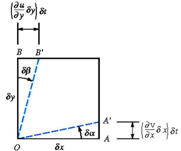
$$\therefore \vec{\omega} = \omega_x \hat{i} + \omega_y \hat{j} + \omega_z \hat{k} = \frac{1}{2} \left[ \left( \frac{\partial w}{\partial y} - \frac{\partial v}{\partial z} \right) \hat{i} + \left( \frac{\partial u}{\partial z} - \frac{\partial w}{\partial x} \right) \hat{j} + \left( \frac{\partial v}{\partial x} - \frac{\partial u}{\partial y} \right) \hat{k} \right]$$
